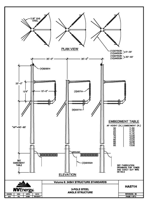
Figure 9: 345-kV Steel Three-Pole Dead-End/Angle Structure
